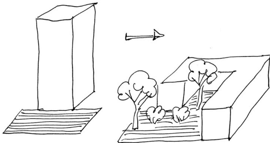
*Figure 3.2. Morphing a tall building's footprint and shape to create a semi-enclosed urban space saves what was psychologically unusable exterior space. The usable interior volume nevertheless remains the same.*
